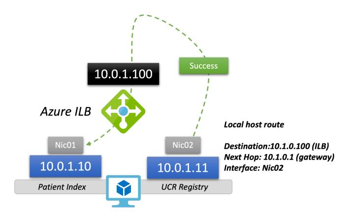
This allows the communication to be successful now that the backend-to-frontend now has a different source (10.0.1.11) and destination IP address (10.0.1.100 > DNAT > 10.0.1.10).
