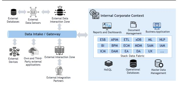
The operation of the data is in Data Intake Gateway, using ESB and API Gateway technology to capture, orchestrate, transform, enrich and integrate data assets into to corporate data assets.
