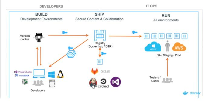
Here we can see the separation of the three main stages:
