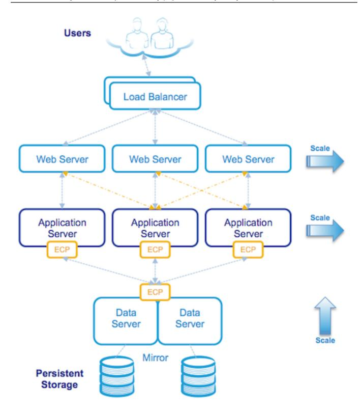
Although at first glance the architecture may look complicated it is still made up of the same components as a Caché system installed on a single server, but with the logical components installed on multiple physical or virtual servers. All communication between servers is via TCP/IP.
